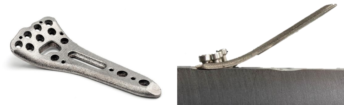
Figure 2: Fixation of the radius plate in the test setup
