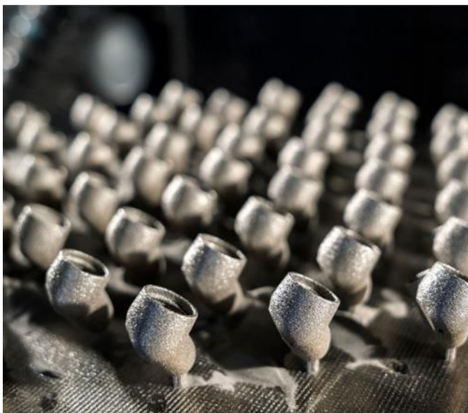
Figure 2: Automated series process in 3D printing via selective laser melting for the production of IE 600 housings
