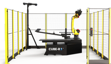
CUBE-R – Mesh and light curtain
