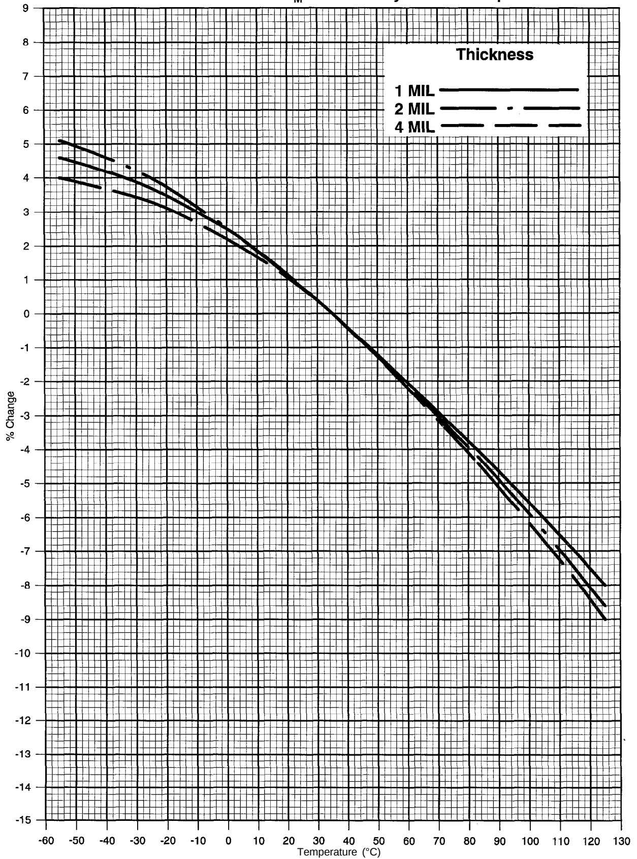
Curve #5: Variation of B_M of Permalloy 80 with temperature
