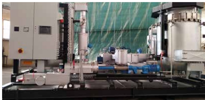
Customers can now test their own lubricant oil formulations on site with EDL's portable LEPD pilot plant. The plant was manufactured by TAF.
