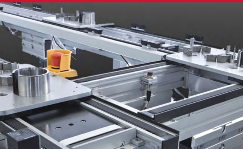
Strecke | transfer line
