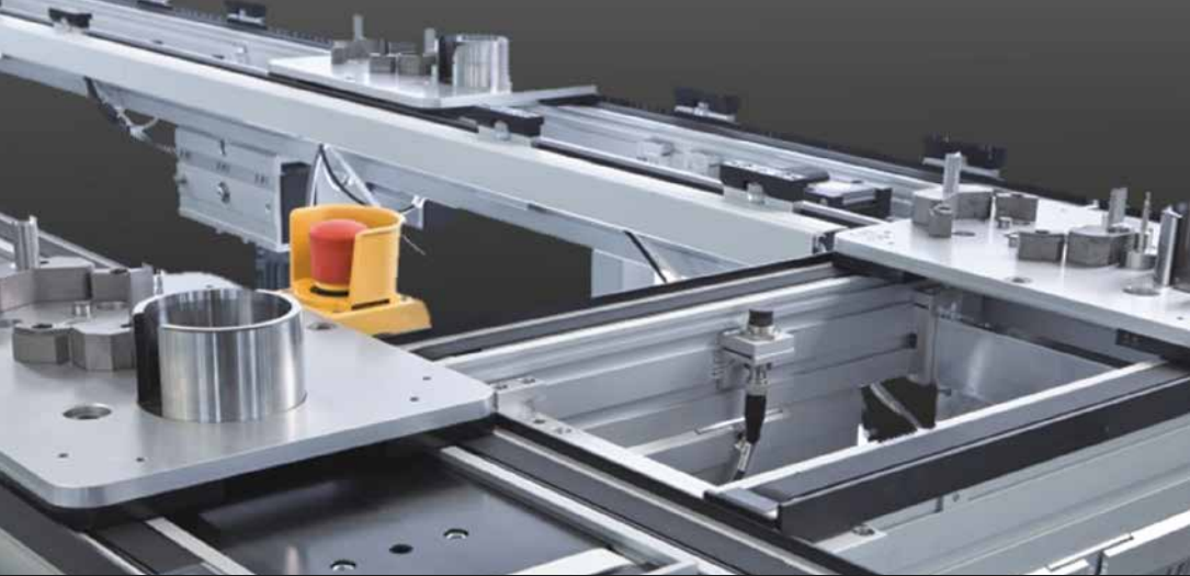
Strecke | transfer line
