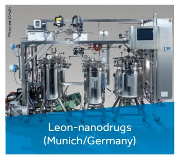
Modular mobile platform for nanoparticles in API production: EPC project, fast track development of the package during 6 months from basic design to delivery; capacity 100 Liter/batch.
