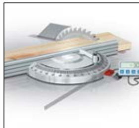
In MagLine Basic, the magnetic band is also used as the system's measuring scale. The flexible design of the magnetic band allows it to be bent to a radius and used for simple angle measurement, e. g. with limit stop systems.
