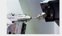
These measurements can be used for initial tool setting, tool replacement cycles, tool wear, tool breakage and thermal growth monitoring.
