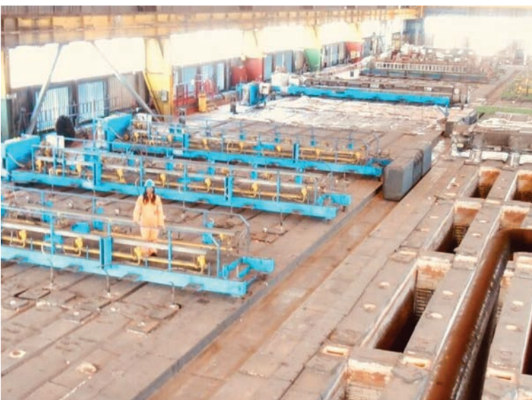
FIGURE 1 Anode baking furnace at Aluchemie.
