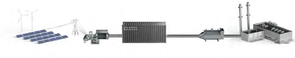
Fig. 12: Schematic of an electrified TES system with resistive heater, storage module and steam generator. Source: Kraftblock.
