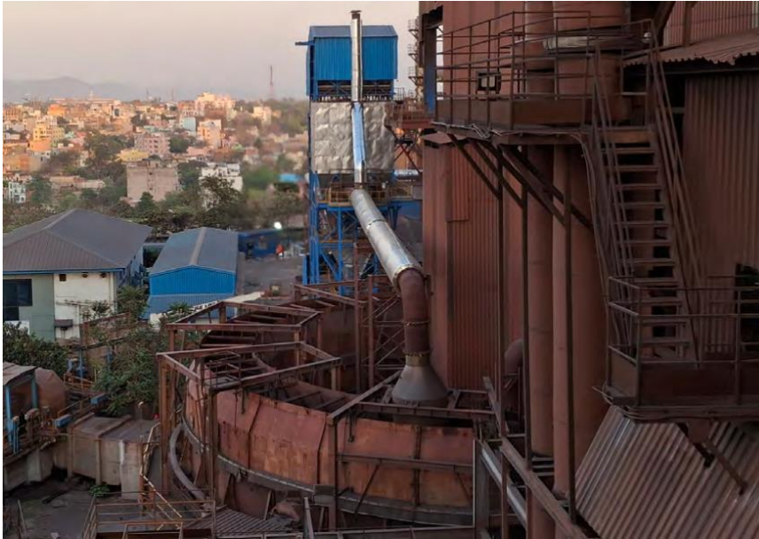
Fig. 10: Hood for waste heat recovery at the sinter cooler of Sinter Plant 3 in Jamshedpur.
