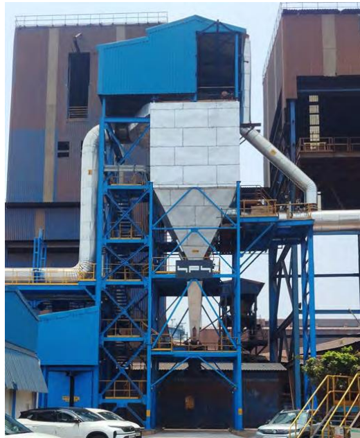
Fig. 10: Hood for waste heat recovery at the sinter cooler of Sinter Plant 3 in Jamshedpur.
